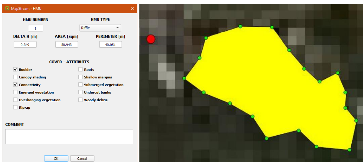
Figure 13: HMU dialog box (left). After clicking the “OK” button a new polygon is added to the HMU shapefile (right).
