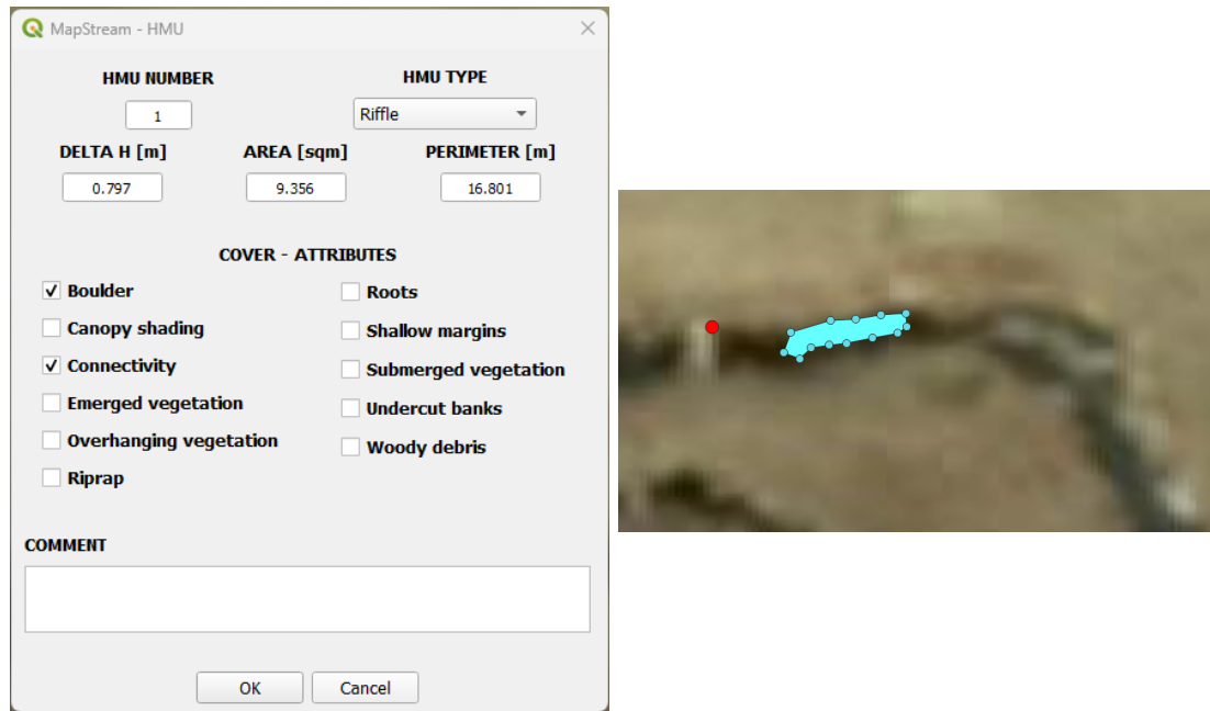
Figure 6.9: HMU dialog box (left). After clicking the “OK” button a new polygon is added to the HMU shapefile (right).
