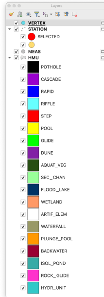
Figure 6.5: Vertex, Station, Meas and HMU shapefiles automatically generated and uploaded into the QGIS Layers panel.
